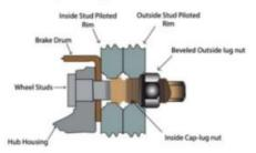
piloted wheel, put two drops of oil on the stud and inside the nut, set the hub so that the pilot face is at the 12 o'clock position and start tightening at that 12 o'clock stud
